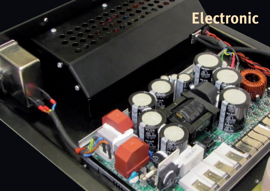
A 500 watt amplifier takes the low frequencies from an active coupler and feeds them to the low-frequency driver.
