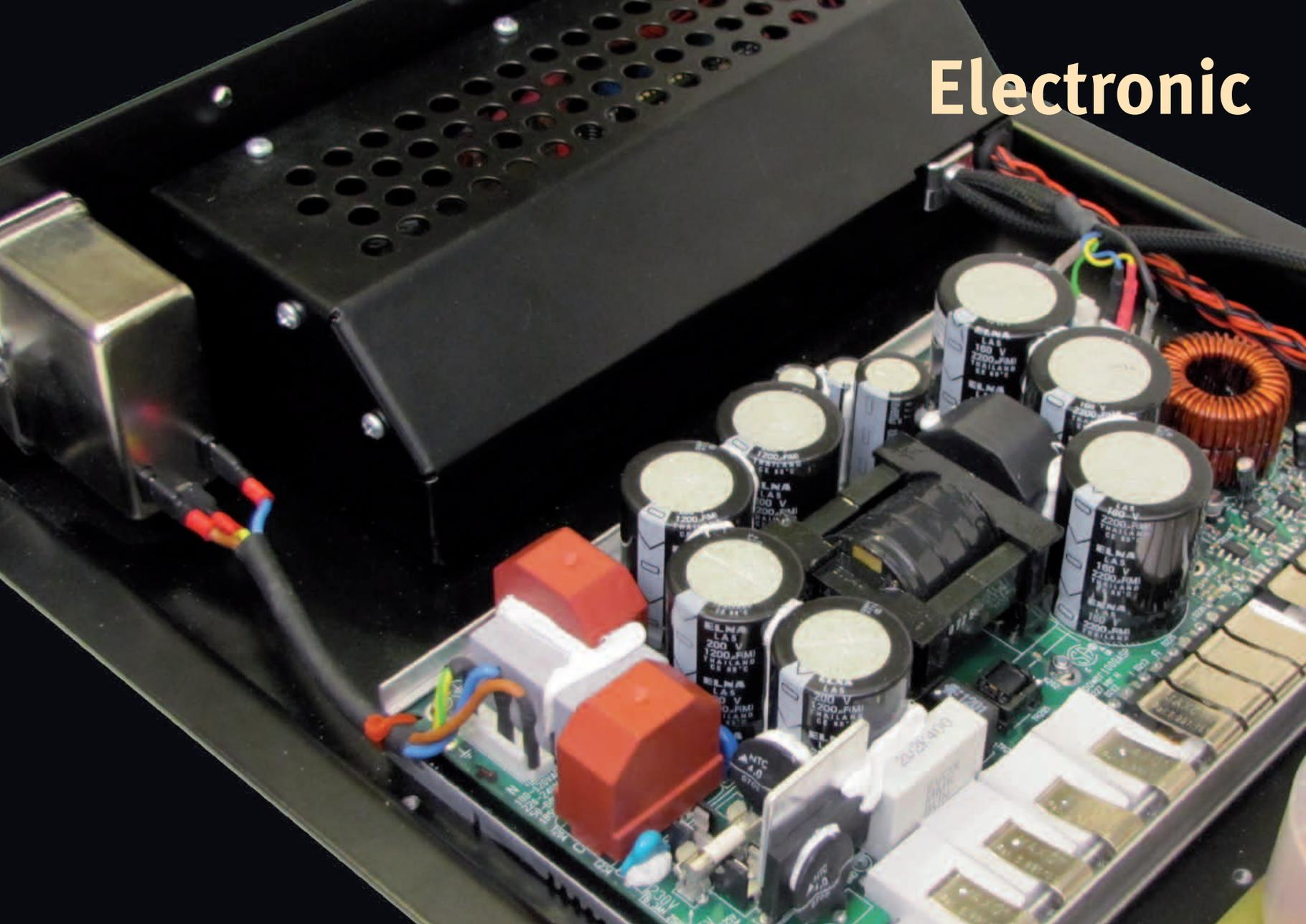
A 500 watt amplifier takes the low frequencies from an active coupler and feeds them to the low-frequency driver. Its circuit topology is designed for minimum output impedance, enabling it to achieve a maximum damping factor, and resulting in absolute control of the bass membrane. The integrated volume control allows for individual adjustment of the bass module to the listening room.
